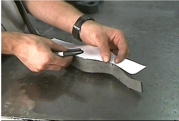
Figure 11 - Front Template Bend Profile
