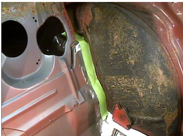
Figure 6 – Cut Line Extension Using 2" Tape
