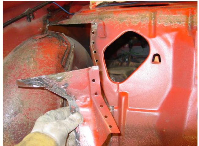
Figure 2 – Seat Support Removed
