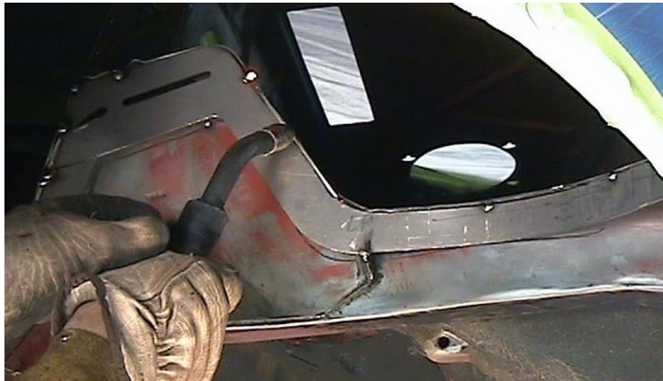
Figure 14 – Tack Weld Tub Flanges
