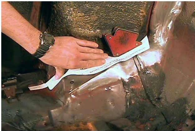
Figure 4 – Inner Wheelwell Front Template
