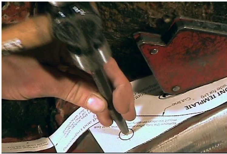
Figure 3 – Inner Wheelwell Front Template with Tab
