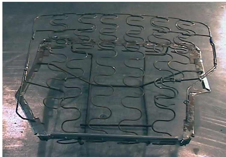
Figure 24 – Narrowed Rear Seat Frame
