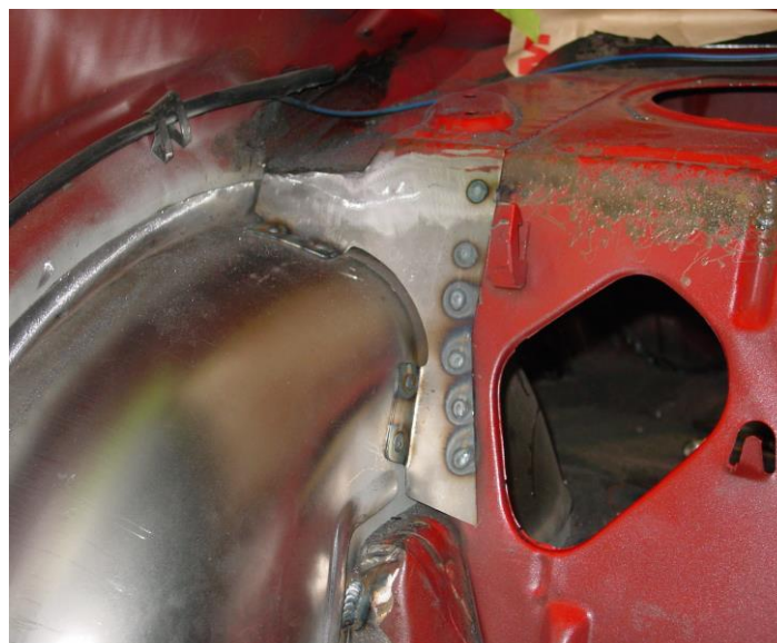
Figure 22 – Seat Back Bracket Installed
