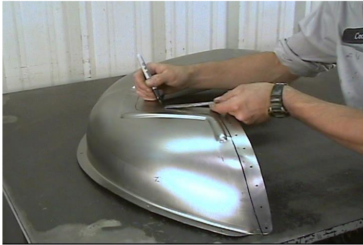
Figure 16 – Mark Tub Mounting Surfaces
