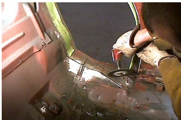
Figures 8 & 9 - Metal Removal for Clearance of DSE Deep Tubs
