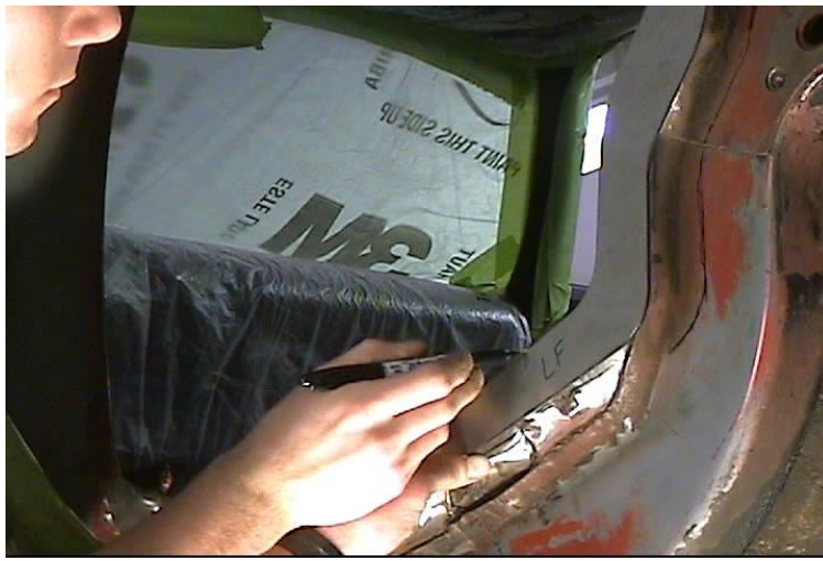
Figure 10 - Front Flange Alignment
