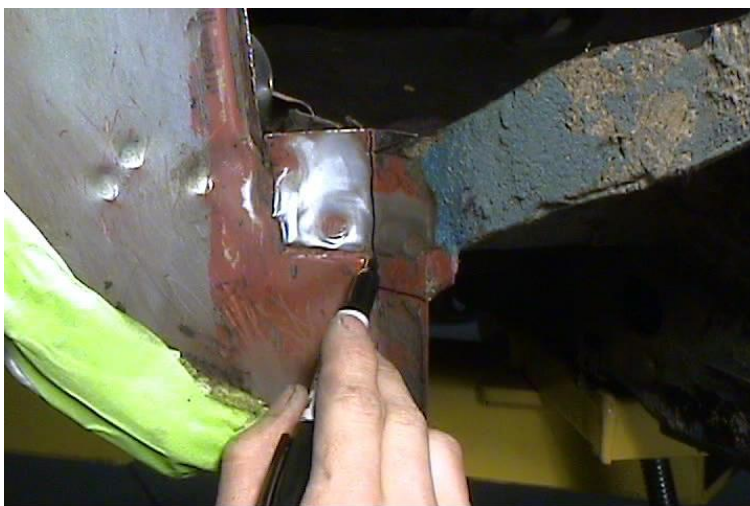
Figure 7 - Marking Tab for Removal
