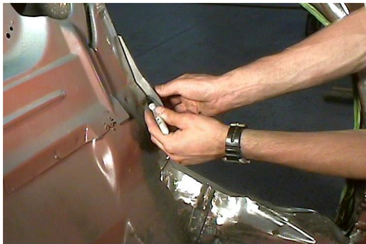
Figure 13 - Marking Front Template to Floor Pan Profile
