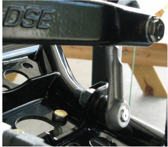
Figure 24 – Attach the Anti-Roll Bar Arm to the End Links
