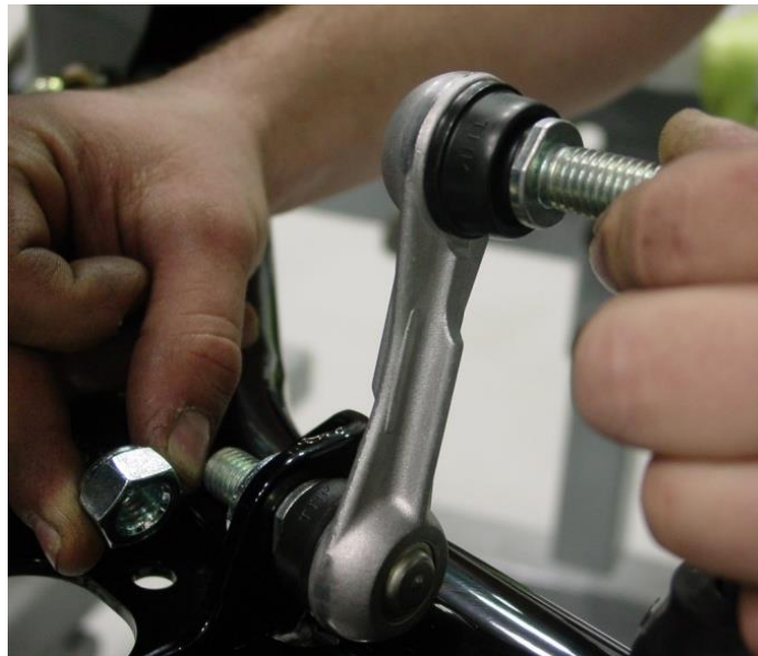
Figure 23 – Attach the End Link to the Lower Control Arm
