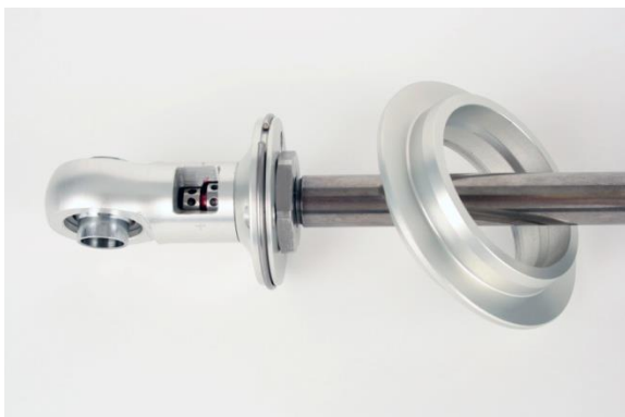
Figure 8 – Removing the Upper Spring Seat
