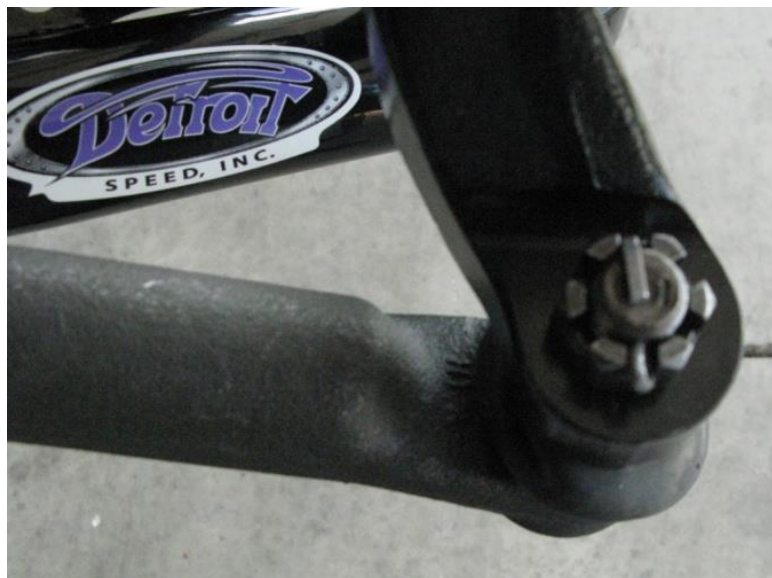
Figure 25 – Attach the Outer Tie Rod to the Steering Arm
