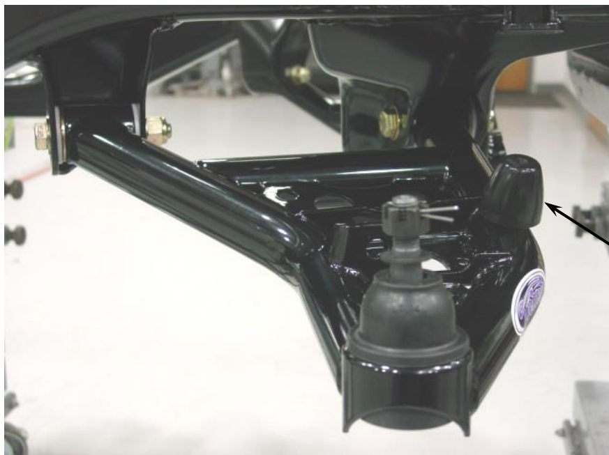
Figure 2 – Passenger Side Control Arm Shown
