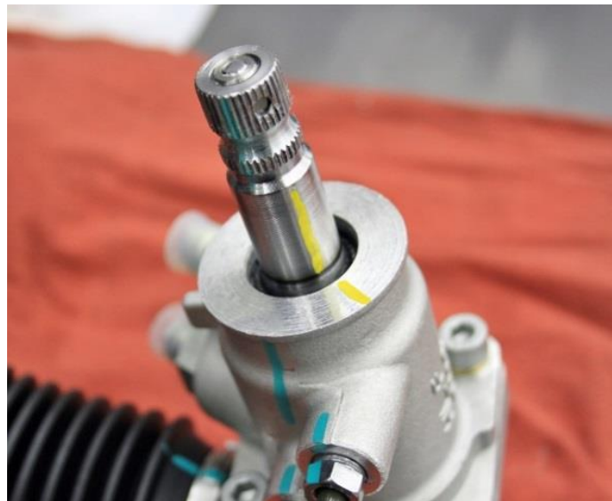
Figure 14 – Center the Rack & Pinion
