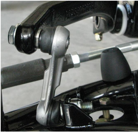
Figure 24 – Attach the Anti-Roll Bar Arm to the End Links
