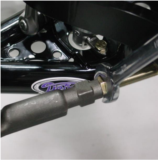
Figure 17 – Measuring the Outer Tie Rods
