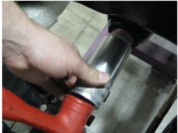
Figure 19 – Fully Installing the Bushings
