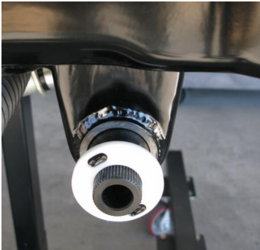
Figure 18 – Installing the Bushing & ARB
