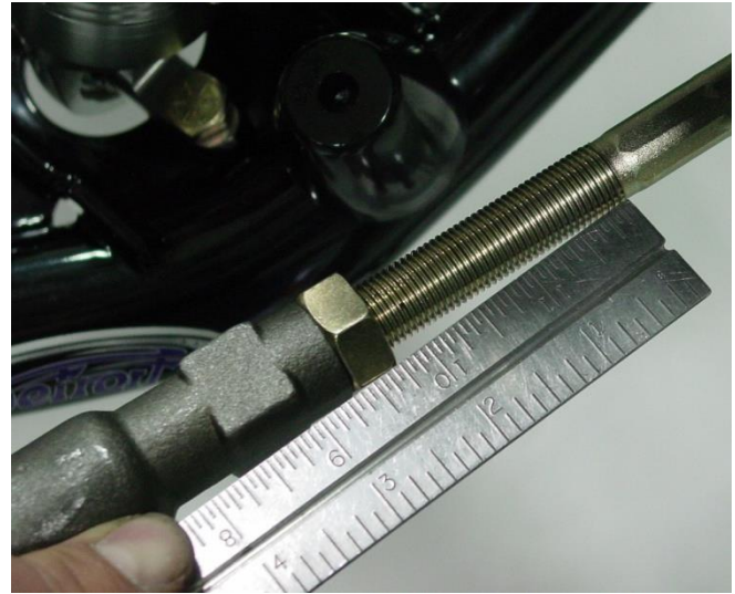
Figure 17 – Measuring the Outer Tie Rods
