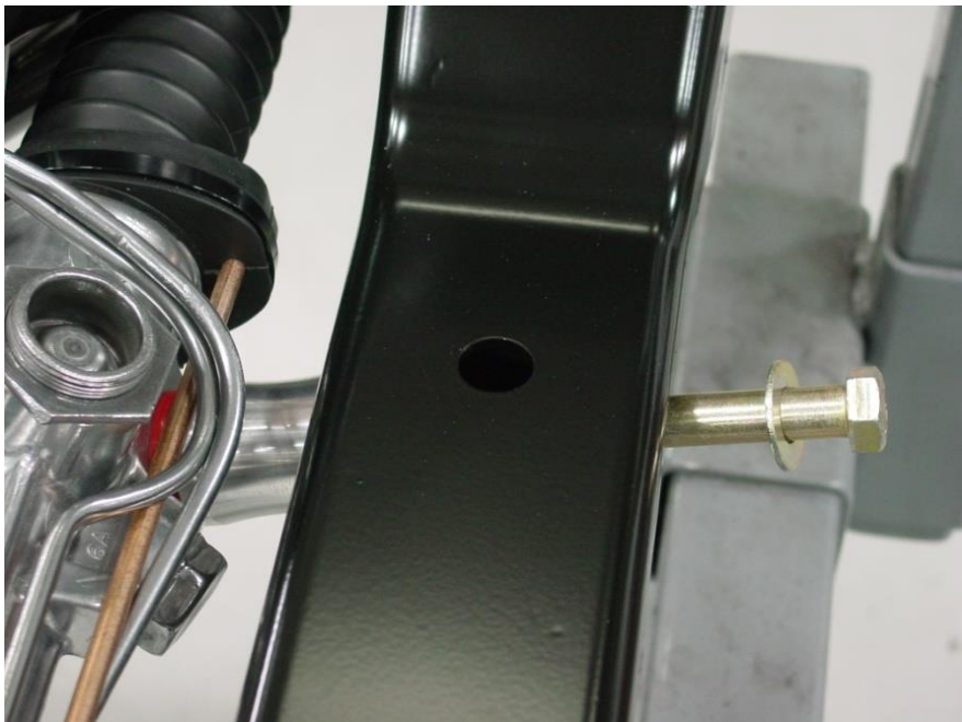
Figure 16 - Attaching the Rack to the Cross Member
