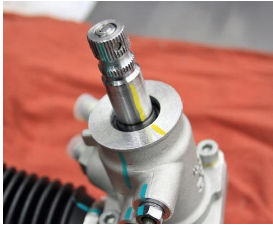
Figure 15 – Center the Rack & Pinion
