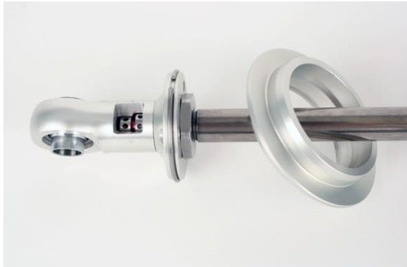
Figure 9 – Removing the Upper Spring Seat
