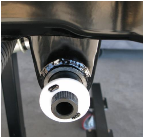
Figure 19 - Installing the Bushing & ARB
