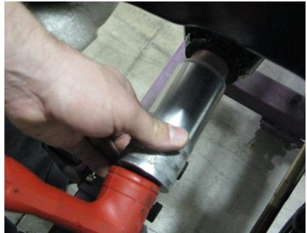
Figure 20 - Fully Installing the Bushings
