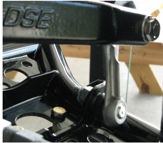
Figure 25 – Attach the Anti-Roll Bar Arm to the End Links
