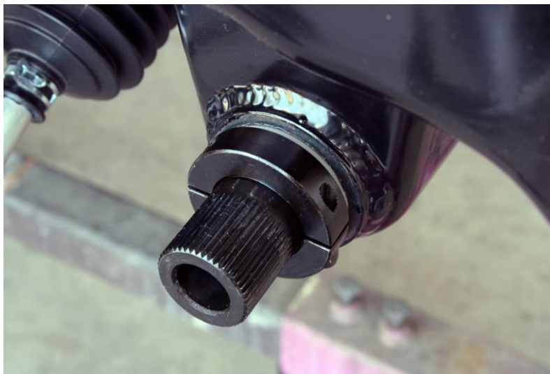
Figure 22 – Indexing the Clamp
