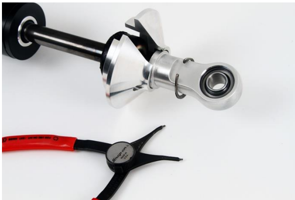
Figure 6 - Removing the Snap Ring
