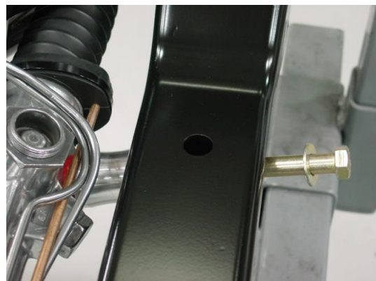
Figure 17 – Attaching the Rack to the Cross Member
