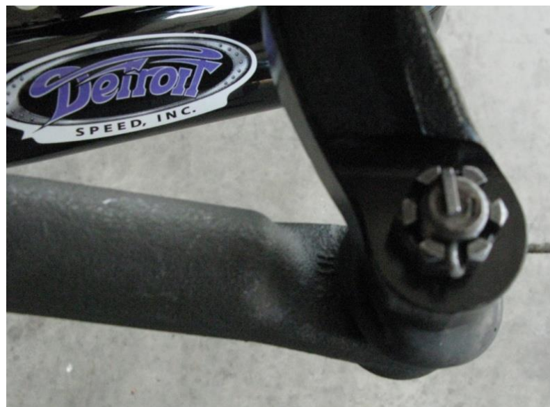
Figure 26 – Attach the Outer Tie Rod to the Steering Arm
