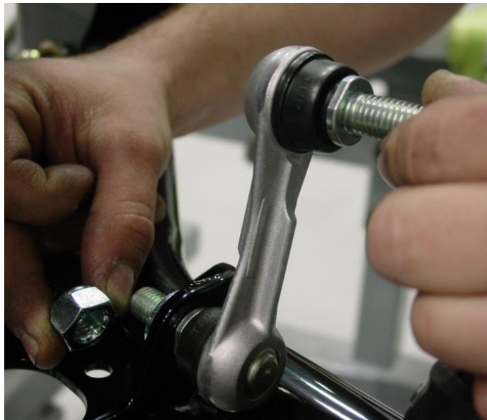
Figure 24 – Attach the End Link to the Lower Control Arm
