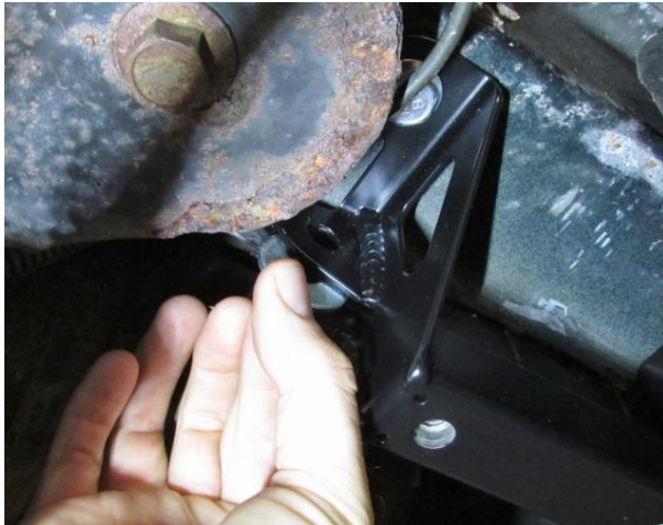
Figure 2 - Install M10 Washers
