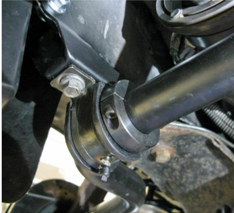
Figure 7 – Install Split Lock Collars
