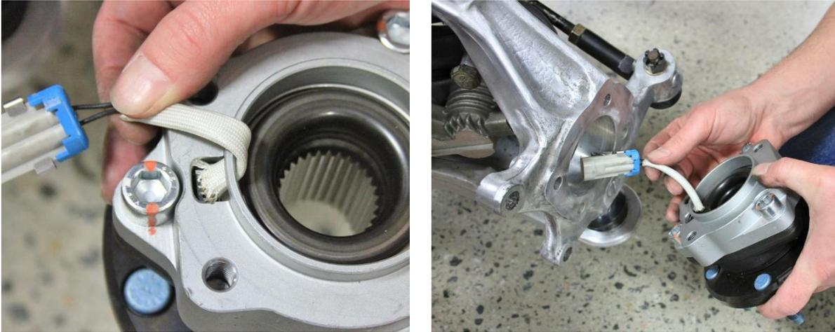
Figure 4 – Position Detroit Speed X-Tracker Hub Assembly (1991-96 Corvette)
