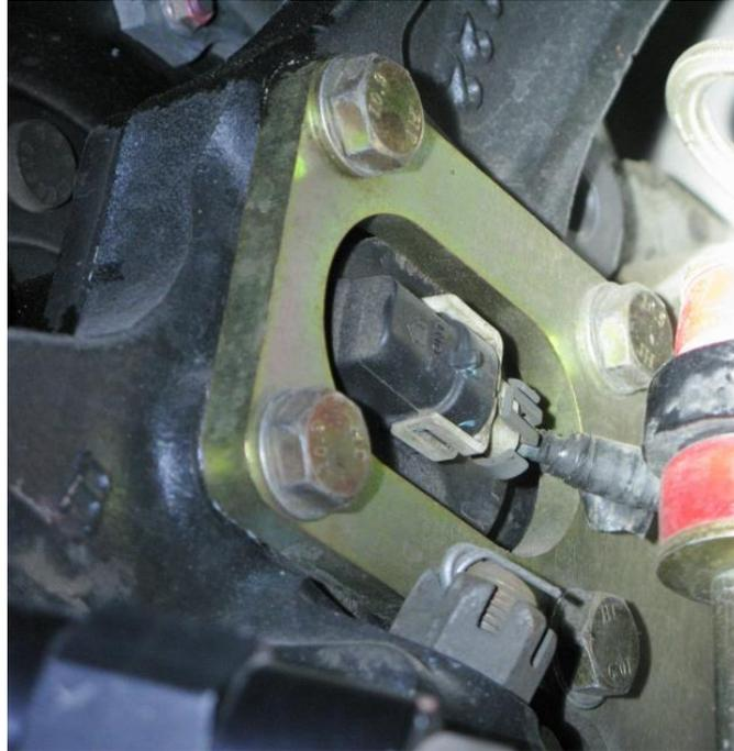
Figure 2 - Unplug ABS Sensor (1993-2002 F-Body)
