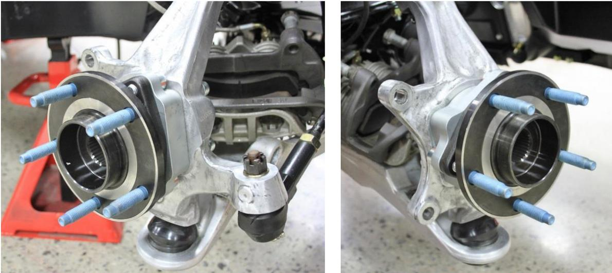
Figure 5 – Install Adapter Assemblies (1991-96 Corvette)
