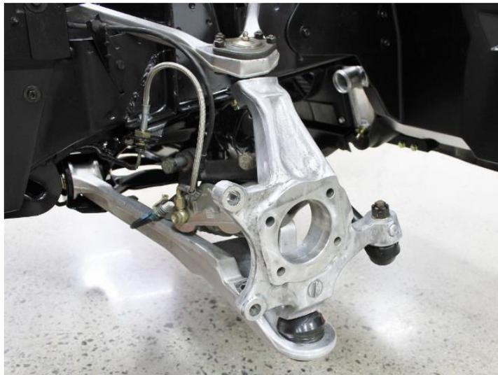
Figure 3 - Remove Factory Hubs (1991-96 Corvette)
