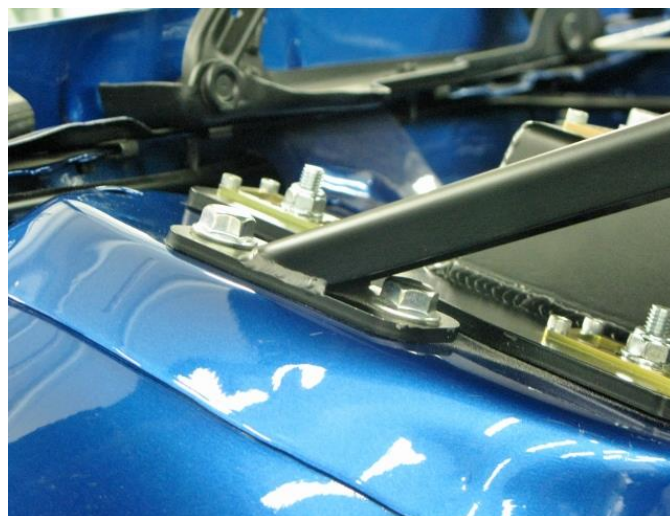
Figure 3 - Install M10 Fasteners
