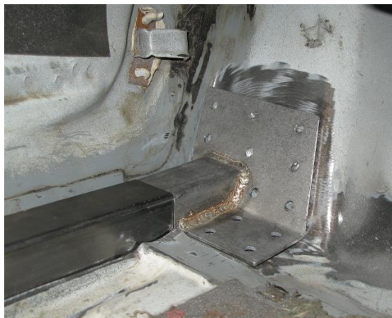
Figure 28 – Front Inner Torque Box Doubler
