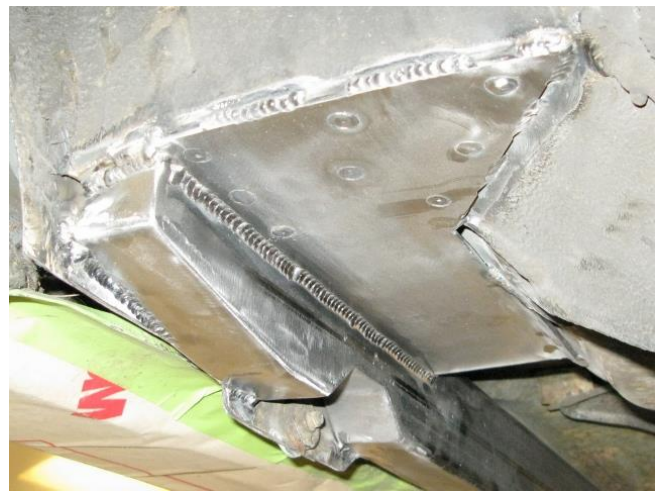
Figure 15 - Finish Weld Doubler & Closeout Plates
