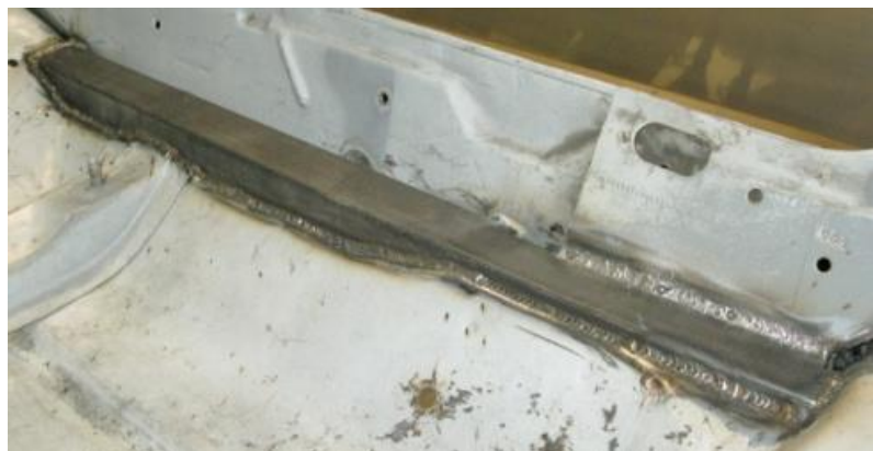
Figure 16 - Finish Weld the Connector
