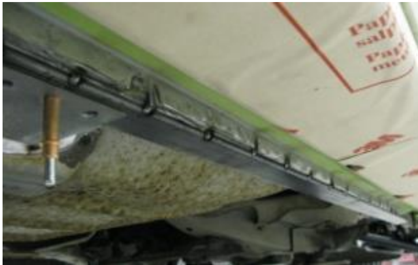
Figure 12 – Tack Weld Connector
