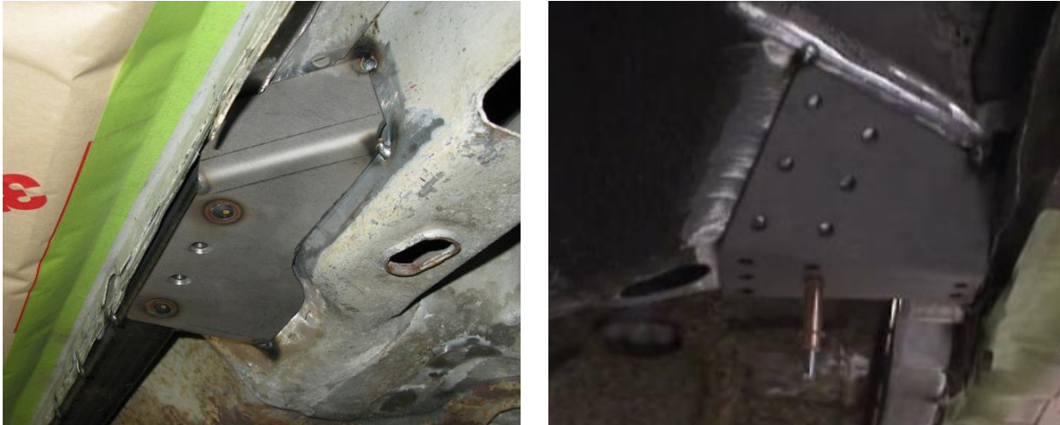
Figure 27 – Tack & Plug Weld Doubler Plates
