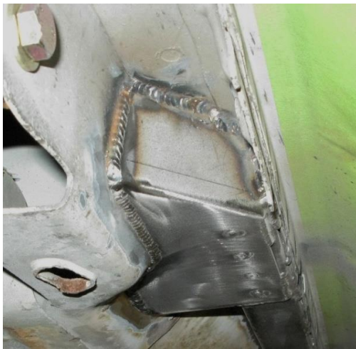
Figure 15 - Finish Weld Doubler & Closeout Plates
