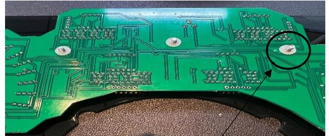
Lay nylon washers over the screw to protect circuit board
