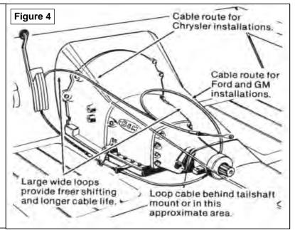
13. Move the transmission selector lever by hand to the full rear position (Low). Operate the shifter lever to the Low gear position (ratcheted all the way back). Adjust the large nuts on the cable so that the swivel will slide into the front hole on the selector lever. Tighten the large nuts completely. Be sure that the swivel will slide freely in and out of the hole in the selector lever.
