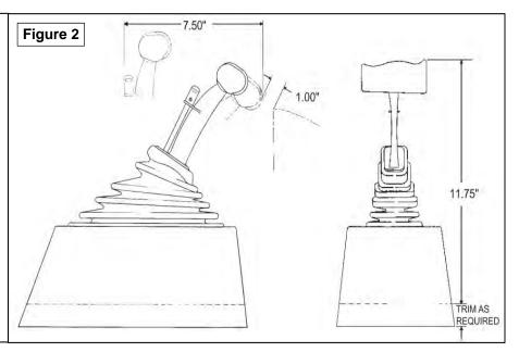
3. Drill four 9/32" mounting holes where marked. Temporarily mount the shifter in place using washers as required to get it level. **Do not bend the mounting brackets on the bottom of the shifter.** Mark the location for the shifter cable hole, 3" ahead of the left front shifter mounting hole. Drill or cut a 1-1/2" diameter cable hole in the floorboard.
