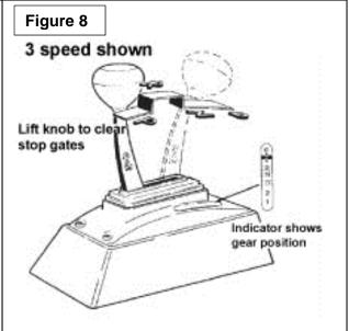
**Park:** To get Park from any straight gate gear position, lift the stick all the way and push the stick all the way forward to the Park position. Release the stick and the shifter is locked in Park. To get to any other gear position you must raise the stick to clear the stop gates.
