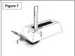
26. Set a pair of dividers at the distance X, measured in Step 25. Holding the tower in position, place one leg of the divider against the floor while the other touches the tower (See Figure 7). Using the dividers, scribe a line around the tower that follows the contour of the floorboard. Remove the tower and trim at the scribe line using tin snips.
