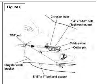
20. Remove the two transmission oil pan bolts directly below the shift lever. Install the cable bracket into position with two spacers between the pan and the bracket (See Figure 6). (If your transmission is equipped with a cast aluminum oil pan these spacers can be omitted). Install the two supplied  $5/16-18 \times 1.00^{\circ}$  pan bolts and tighten to 12-13 lb. ft. Do not overtighten as this can damage the pan gasket.
