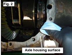
9. We recommend running a 5/16"-18 or M8x1.25 (some applications have metric fasteners) tap through each threaded cover hole on the axle housing to ensure an accurate torque on all bolts.
