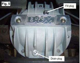
17. Fill with factory recommended gear oil using the B&M Cast Aluminum Rear End Cover fill plug hole (See Figure 5). Add gear oil until oil runs out of the axle housing fill hole.
