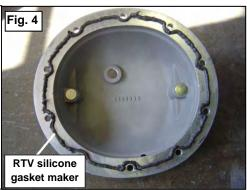
12. Install the B&M Cast Aluminum Differential Cover on the axle housing using a supplied bolt and washer at a bottom hole on the cover so it can be used as a guide.
