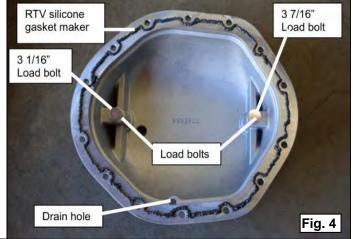
12. Install the B&M Cast Aluminum Rear End Cover on the axle housing using a supplied bolt and washer at a bottom hole on the cover so it can be used as a guide.
