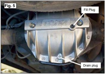
17. Fill with factory recommended gear oil using the B&M Cast Aluminum Rear End Cover fill plug hole (See Figure 5). Add gear oil until oil runs out of the axle housing fill hole.
