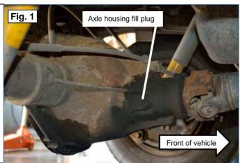
4. Remove all the bolts from the cover except one at the top. Loosen the remaining bolt but do not remove.
