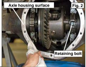
9. We recommend running a M8-1.25 tap through each F threaded cover hole on the axle housing to ensure an accurate torque on all bolts.
