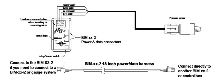
This Bus Interface Module connects to a solid state pressure sensor. There are two power & data interface (I/O) ports on the module. Either one can be connected to the gauge system or to another module, allowing several units to be daisy chained together. Do not connect the I/O port to anything other than a Dakota Digital gauge or BIM. Do not mount the module in the engine compartment; it should be mounted in interior of the vehicle.
