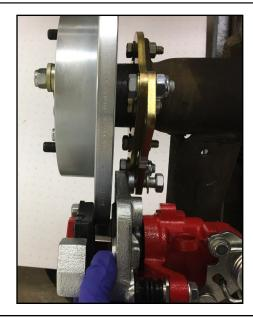
**8.** Next install the correct side caliper (Bleeder always points up). Use the supplied 12x30mm hex bolts and washers to secure the caliper.
