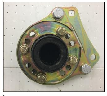
**3.** Install the intermediate steel bracket to the inboard side of the base steel bracket as shown using the supplied 12x30 hex bolts. Make sure the 12mm nylock nuts are installed inboard. Torque the nylock nuts to 85ft lbs
