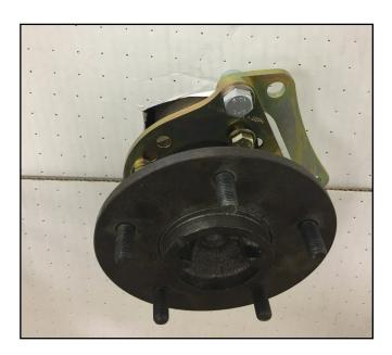
**5**. Next re-install the axle, c-clip, pin, retaining bolt and cover. Now is a good time to check your wheel seal for wear. Replace if necessary. If all is good, torque the differential cover to the manufacturers specs.
