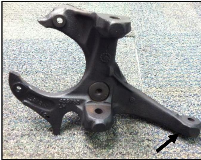
**Figure 1:** Strike tie rod end boss here with large hammer
