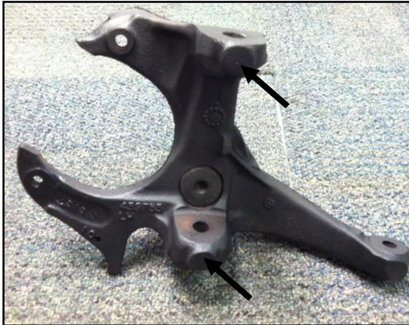
**Figure 2:** Strike here to dislodge ball joints
