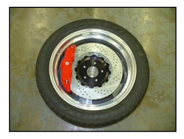
• When installing new Baer rotors, be sure to follow the direction of rotation indicated on the rotor hat area with either an arrow, or an "L" for left, or an "R" for right, or both. "L" or left always indicates the driver's side of US spec vehicles. Images shown are "L" left rotors:
