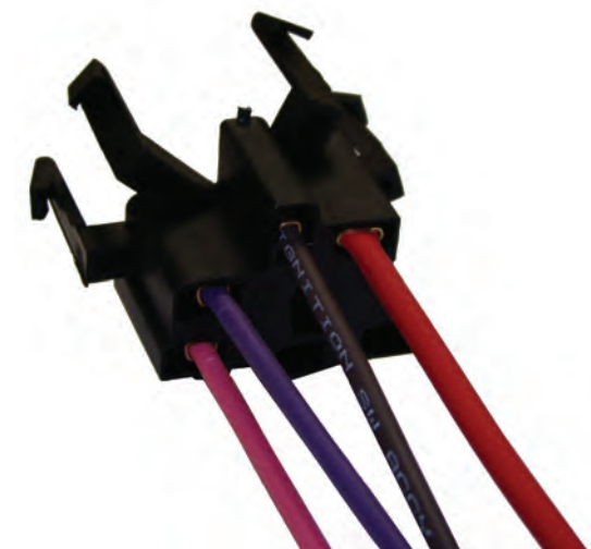
1968 ignition switch connection
