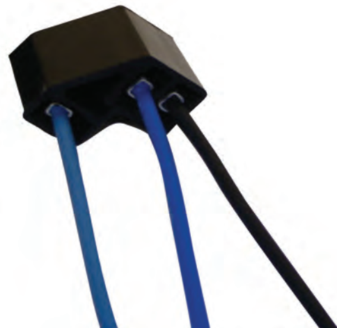
1968 wiper switch connection with depressed park
