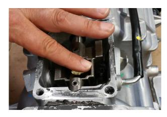
9. Apply a bead of RTV to Seal shifter flange before mounting.
