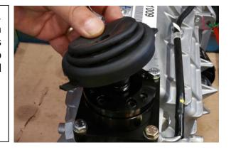
Position the offset stub onto the shifter and make sure that it is offset towards the driver's side as seen in the photo. Secure the offset stick with the provided 3/8"-24 Button Head bolt and washer and torque to 35 ft/lbs.
