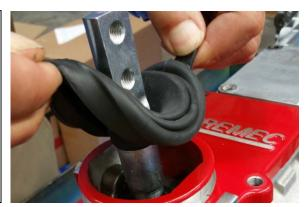
The shifter "body" will be in the in the forward position on the rear T56 shifter cavity. Make sure the pivot ball is positioned into the rear socket and that the white plastic bushing is still in place.
