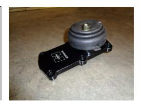
The shifter "body" will be in the in the forward position on the rear TKO shifter cavity. Make sure the pivot ball is positioned into the forward socket and that the white plastic bushing is still in place.
