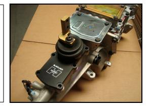
Attach the Chrome Hurst shift handle to the lower stub stick using the supplied hardware. This shifter locates the handle in nearly the same location as the stock shifter hole in the floor. There may be some modification required to the floor or tunnel area to accommodate the larger size of the Tremec transmission.
