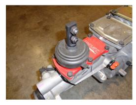
The shifter boot that is included with the stock Tremec shifter can be re-used on the Hurst shifter. To use this boot, it will need to be modified by cutting off the bottom section of the boot as shown.
