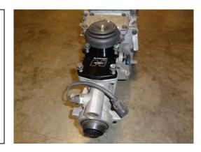
Position the offset stub onto the shifter and make sure that it is offset towards the driver's side as seen in the photo. Secure the offset stick with the provided 3/8"-24 Button Head bolt and washer and torque to 35 ft/lbs.
