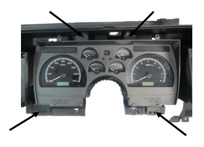
7. Re-install the gauge cluster bezel and lower panel to the dash using the factory hardware and refer to the main manual for wiring instructions to complete the VHX installation.
