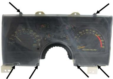
The inner gauge panel and column dust seal will be reused so remove the six (6) screws that secure the clear lens and also the additional three (3) screws on top that mounts the inner gauge panel. Save all hardware for reassembly.
