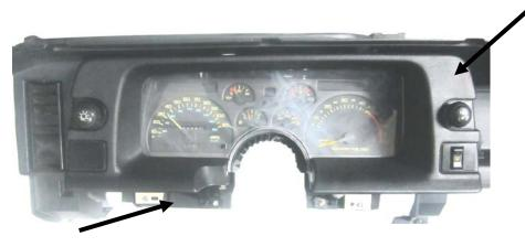
Remove the stock gauge cluster from the dash by removing the four (4) screws, retain the hardware for reassembly.
