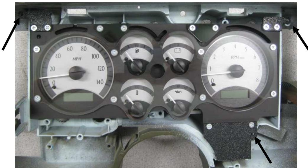
7. Separate the stock lens from the blackout plate; the original lens is not needed. Place the blackout plate over the Dakota Digital gauges while aligning the mounting holes. Attach the VHX system using the five factory screws. Place the included 1/8" white plastic spacer beneath the blackout plate at the lower-most mounting hole before installing the screw (white arrow).
