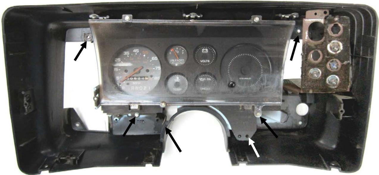
3. Remove the factory gauges by removing the screws shown in the picture below. Your cluster may vary depending on the factory equipment.
