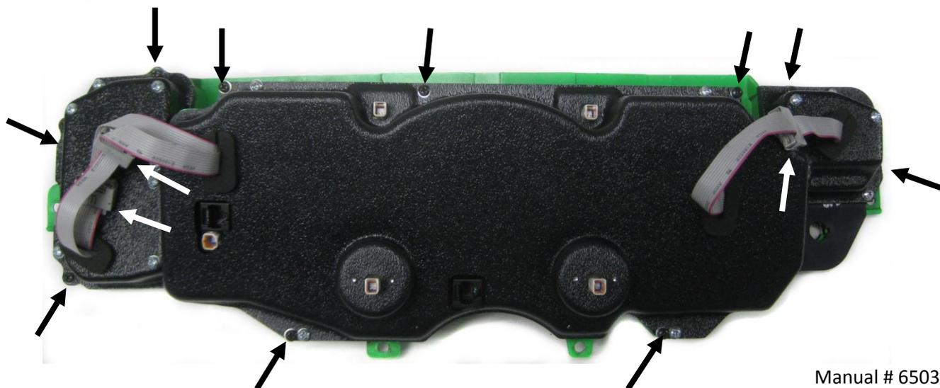
7. Connect the 3-pin wire harness into the clock (white arrow, below) and refer to the included VLK 350360 manual for wiring instructions, and then connect CAT5 cables to the two ports and carefully route the other ends to the control box mounting location.
