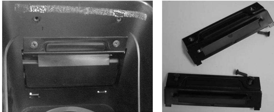
3. Now, remove the light bulbs and indicator light panels. Since these functions are built into the VHX system, you can rewire the indicator wires to the control box to retain the desired indicators.
