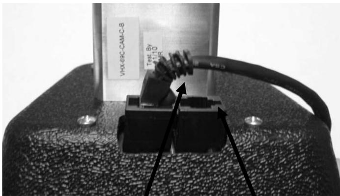
Pre-bend cable to side before installing so unit will sit flush once inserted into dash
