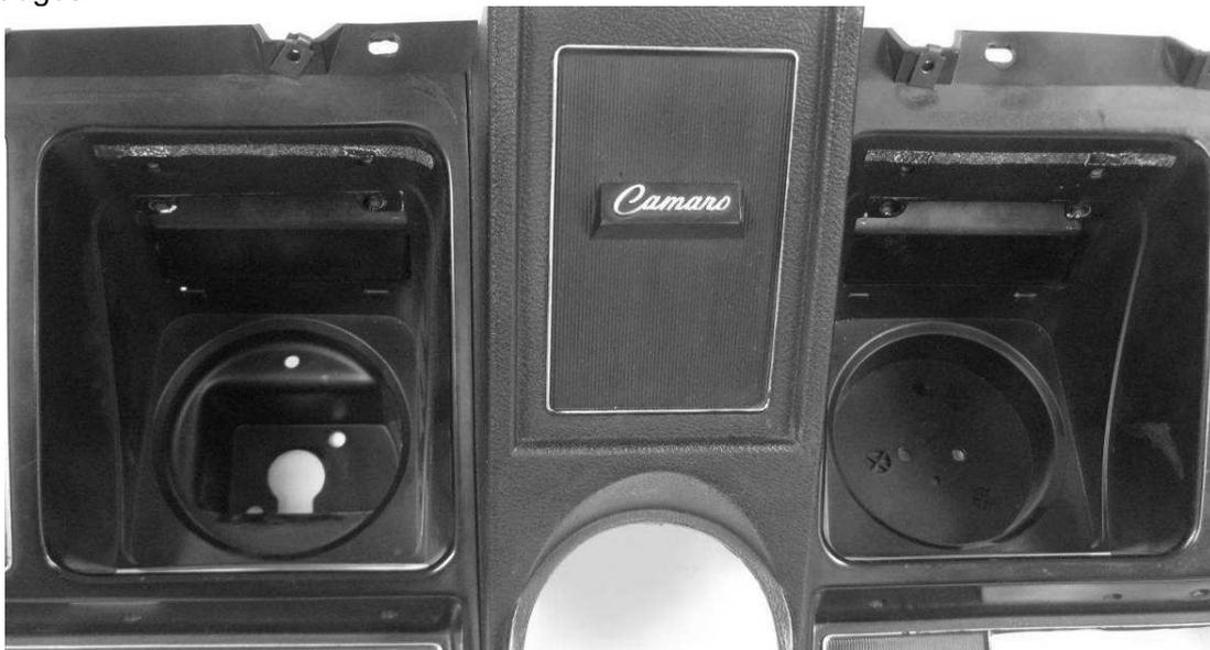
5. Begin with the speedometer installation first; located in the left side opening in the factory dash. Cut three pieces of the supplied foam tape, 2" long. Install foam strips on the top and sides of each opening about 1/2" down from the face of the housing. This foam provides a cushion where the new VHX cans are installed and forms a tight, rattle-free fit.
