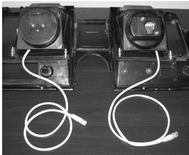
11. As the system is installed, route both CAT5 cables to the control box and connect them to two of the three jacks on the control box. It doesn't matter which cable goes where, all of the jacks are the same.
