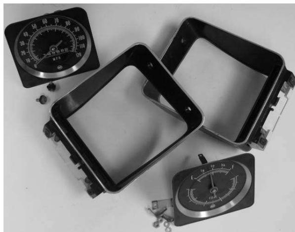
2. Once the original gauge internals have been removed, there are two reflectors (one on each side) inside the housing that need to be removed for clearance of the new VHX gauges (see photo).
