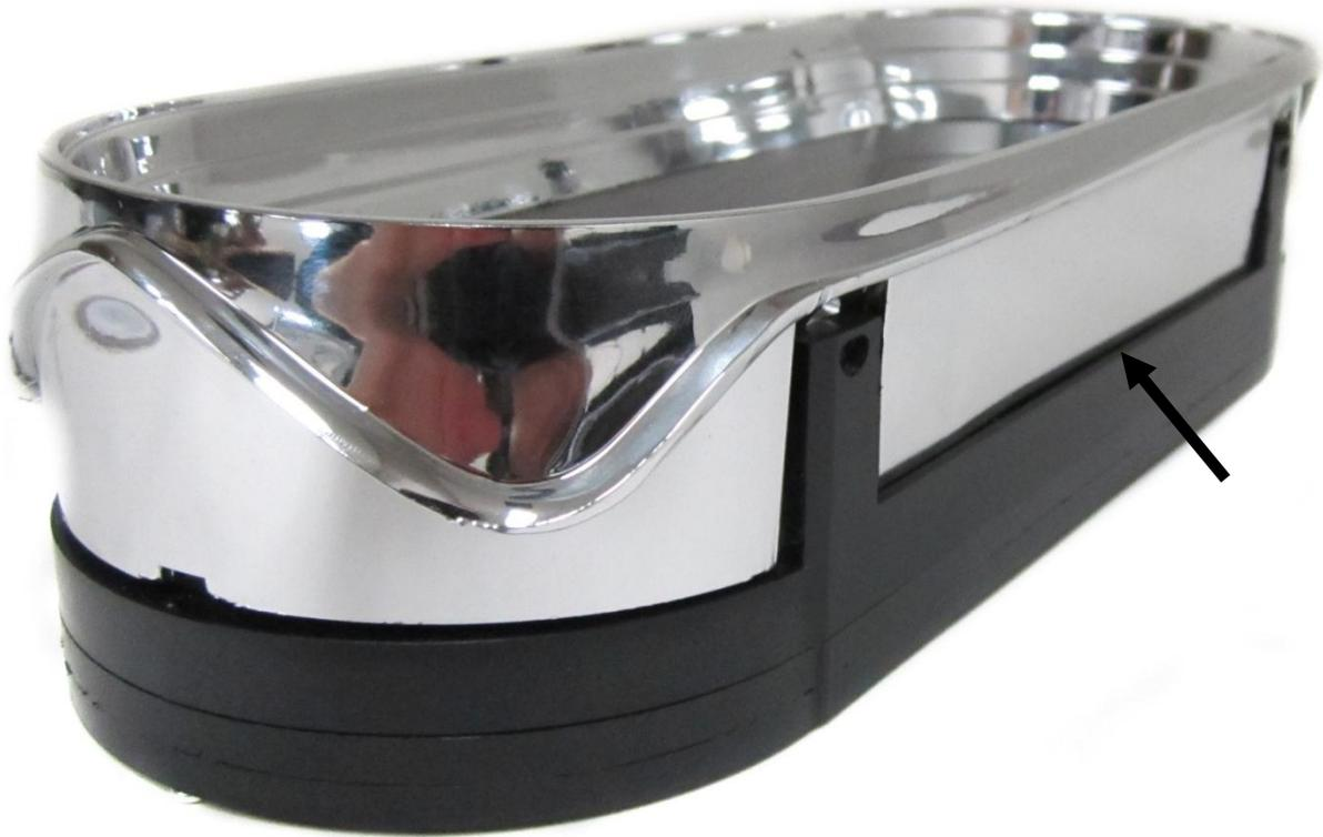
4. To attach the bezel to the VHX system, use the four (4) screws provided. Use the smaller 6-20x1.75" for a stock bezel or the larger 8-18x1.75" for a reproduction bezel.
