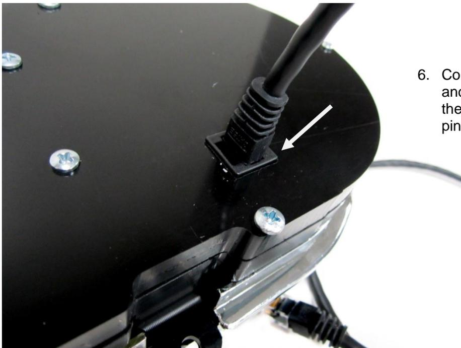
6. Connect the CAT5 cable to the backside and take care when routing this cable to the control box mounting location to avoid pinching the cable.
