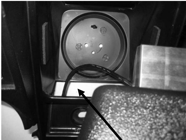
Cable routed through indicator light opening
