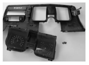
3. Remove the stock gauges from the stock lens spacer. The lens spacer is going to be reused to secure the new VHX gauges to the dash/bezel. Remove seven screws holding the gauges to the spacer. Save the screws, they will be reused to attach the new VHX system.
