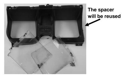
5. This step is optional for automatic transmission bezels only. If you purchased a separate GSS-2000 kit from Dakota Digital, the gear position can be displayed in the VHX message centers, therefore the stock gear position indicator can be removed.
