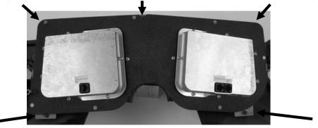
8. Connect the short CAT5 cable between the two gauge housings, then connect the long cable to the system so it can be routed and connected to the control box as the system is re-installed.
