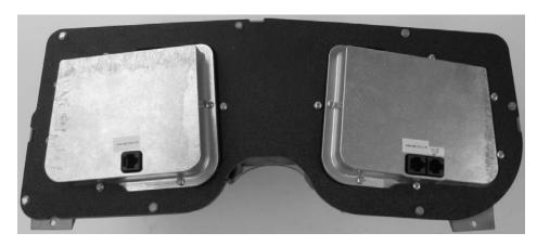
7. Secure the VHX system onto the bezel with the five screws that were removed in step 2.
