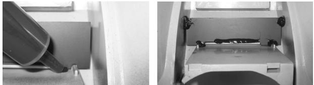
\*\*\* Allow the glue to dry before continuing with the installation.
