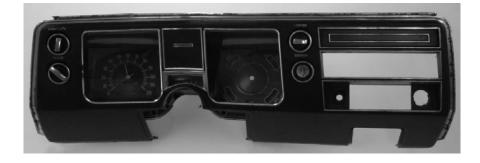
2. Remove the five screws holding the gauges to the bezel as well as the two screws holding ground straps on the back of the system. Save the screws as they will be reused to secure the new VHX system in the steps\_below.
