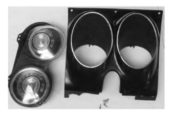
4. For this step, you can re-use the stock foam blocks or use the supplied foam to make replacements for missing or brittle foam pieces. Cut the supplied foam into four small pieces, approx 1.5" long. There are four bosses molded in the bezel where the foam should be placed to help prevent any rattles of the lens and bezel.
