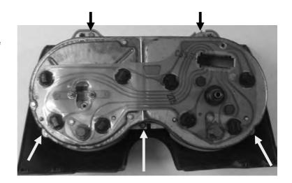
3. Remove the stock gauges and lens from the bezel.
