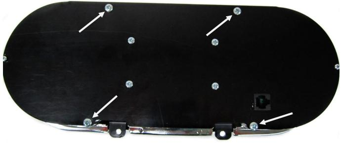
5. Before tightening the screws, double check that the VHX system lens is fully seated and is tight to the bezel.
