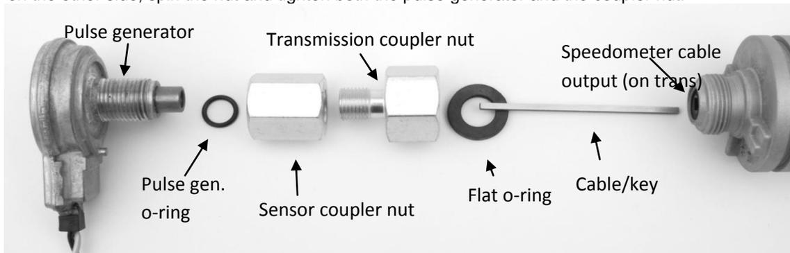
"Exploded" view of sensor install
