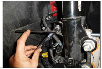
18. Remove the spindle assembly nuts from the bolts only. Do not turn the bolts.
