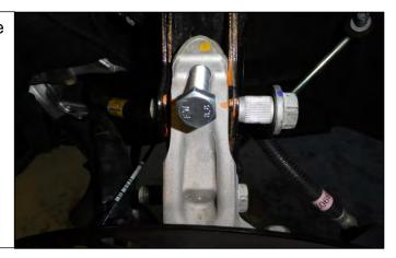
20. Loosen but do not remove the three upper strut assembly bolts from the strut tower.
