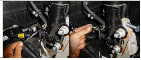
17. Remove the upper sway bar link using a box end wrench with an allen wrench. Once the nut is removed, slide the threaded end of the sway bar link out of the strut assembly.
