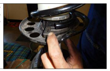
29. To ensure proper spring installation, make sure the Hurst logo is facing up like the image shown.
