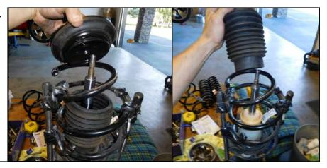
27. Remove the spring. Carefully loosen the spring compressors until they can be removed from the spring.
