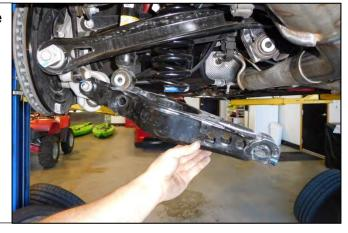
9. Once the spring moves freely, remove the jack and let the rear control arm swing out of the way, while holding onto the spring.
