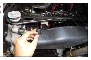
3. Support the rear control arm with a screw jack or Hydraulic jack.
