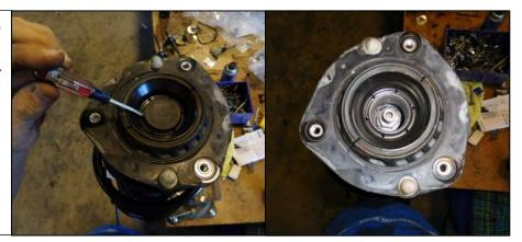
24. With the strut assembly supported, use spring compressors to remove tension from the upper cup of the strut. Springs are under extreme tension. Great care should be taken to ensure safety. If using compressors like the ones shown in the image, tighten them evenly from side to side.
