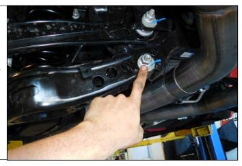
7. Remove the inner control arm bolt. This is a keyed bolt and washer.
