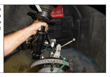
23. Remove the rubber cap from the top of the strut, exposing the nut. The nut will be removed in a later step.
