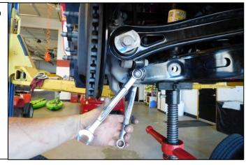
6. Make an alignment mark on the inner rear control arm washer and control arm.
