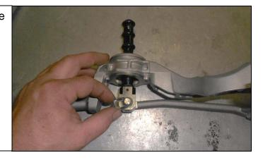
36. Apply a liberal amount of grease to the factory pins that that connect the shifter housing and shift rod to the transmission.
