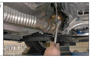
10. Loosen the 15mm nut from the right side exhaust flange connected to the catalytic converter. Spread the clamp open.
