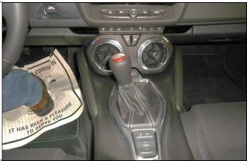
2. Using a trim tool, pry up on the back of the chrome bezel.
