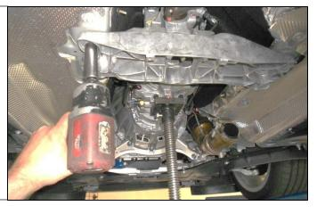
24. Lower the rear of the transmission enough to gain access to the front of the shifter housing.
