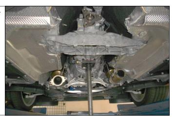
23. Remove the four 15mm bolts from the transmission cross member
