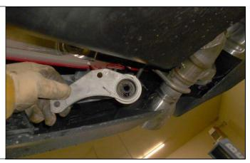
13. The right front exhaust flange is a ball socket you can pry between the transmission cross member and the exhaust to pop it out.
