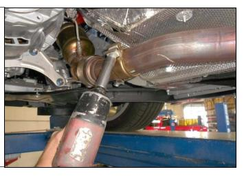
11. Remove the forward rubber isolators from the exhaust system on the left and right side.
