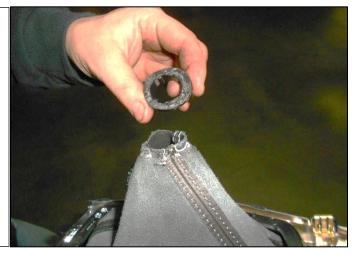
41. With the boot inverted, install the Hurst pistol grip shifter through the boot.
