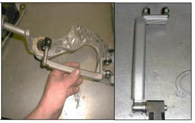
35. Verify that the factory shift rod is oriented in the same position as when it was removed.
