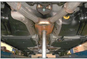
9. Remove the two 15mm nuts attaching the left side exhaust flange to the catalytic converter.
