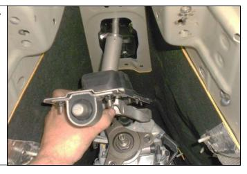
30. Remove the spring clip from the factory shift rod and remove the rod. Take note of the shift rod orientation.
