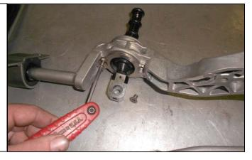
34. Apply grease to the shoulder part of the shift rod. Install the factory shift rod into the pivot block located at the base of the shifter assembly. The pivot block should offset to the right of the shift rod as shown.
