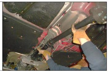
22. Support the transmission with a screw or hydraulic jack.
