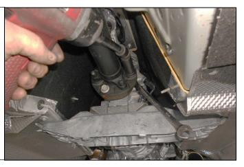
19. Remove the three 18mm bolts and nuts from the flex coupling and differential flange.
