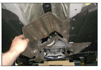
17. The drive shaft must be removed. Start by making an alignment mark on the flex coupling and the transmission flange.
