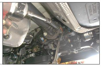
20. Support the drive shaft. Remove the two 15mm bolts from the center carrier bearing. This will allow the drive shaft to be removed from the vehicle.
