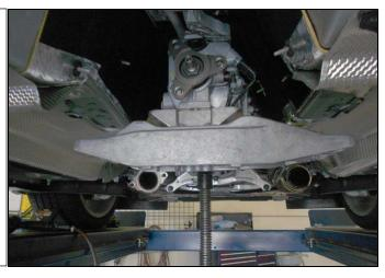
25. The shifter housing is connected to the transmission with a pin on the left and right side. The pin has a spring lock at the end of it as shown here.
