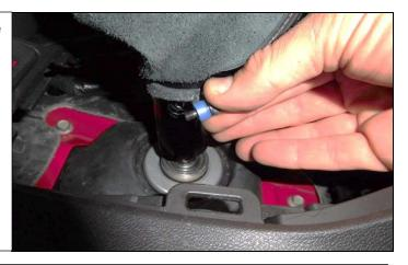
45. Install the shoulder bolts into the pistol grip. Using an 1/8" allen wrench, tighten the shoulder bolts into place.
