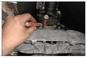
18. Remove the three 18mm bolts and nuts from the flex coupling at the transmission.
