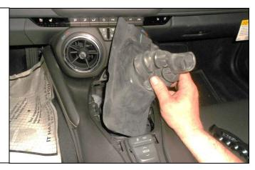
6. Using an extension and 10mm socket, remove the 4 bolts attaching the rubber boot to the transmission tunnel.
