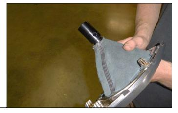
42. Ensure that boot is past the machined groove on the pistol grip and is orientated in the right direction. Secure the shift boot to the pistol grip using the supplied tie wrap.
