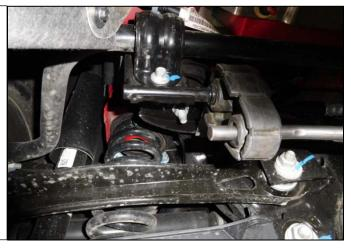
15. Remove the four 13mm bolts from the tunnel brace and remove the brace.
