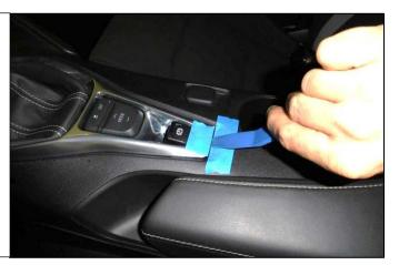
3. Raise the chrome bezel high enough to gain access to the T25 Torx bolt that mounts the shift knob. Remove the bolt.
