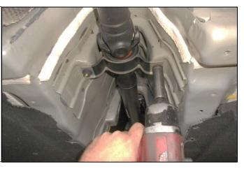
21. The drive shaft can be squeezed together in order to clear the transmission and differential flange.
