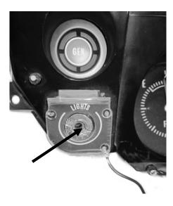
3. Using a large flat head screwdriver or a quarter, remove the screw that secures the headlight switch to the bezel.
