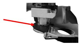
6. Install the Dakota Digital gauge clusters using the included 5/8" screws. All of the stock screw holes will be used. Also make the connections for the auxiliary gauges to their respective length ends.
