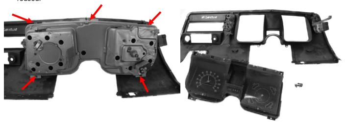
3. Remove the seven screws that hold the stock gauges to the lens spacer. Save this hardware as it will be reused.
