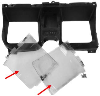
5. This step is optional for automatic transmission bezels only. If you purchased a separate GSS-2000 kit from Dakota Digital, the gear position can be displayed in the HDX message centers; therefore the stock gear position indicator can be removed.
