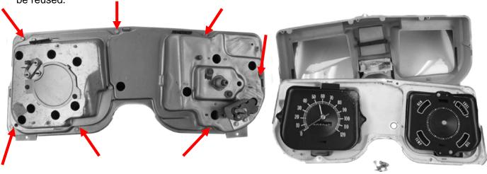
Remove the stock lenses from the lens spacer by removing three screws from the front of each lens. The stock lenses are removed since the new HDX kit features hard coated clear lenses.
