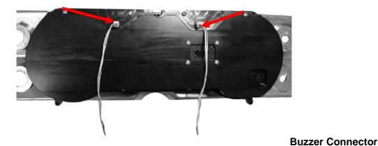
5. Connect the provided Main Harness and the Buzzer (optional for audio feedback) to the back of the HDX system.
