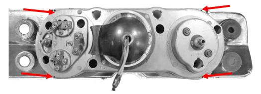
3. Secure the HDX system to the bare bezel using the supplied screws.
