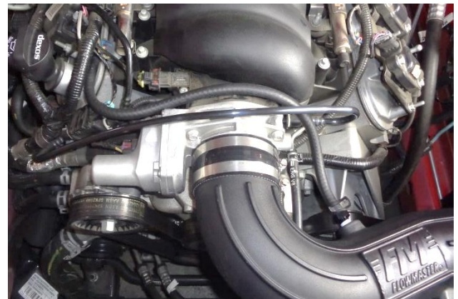
23. Route the hose across the top of the throttle body, below the hard plastic line, and to the barbed fitting. Cut the hose to length, and use the pinch clamp (28) to secure it to the fitting.
