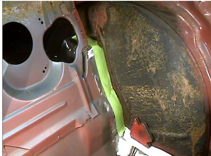
Figure 6 - Cut Line Extension Using 2" Tape
