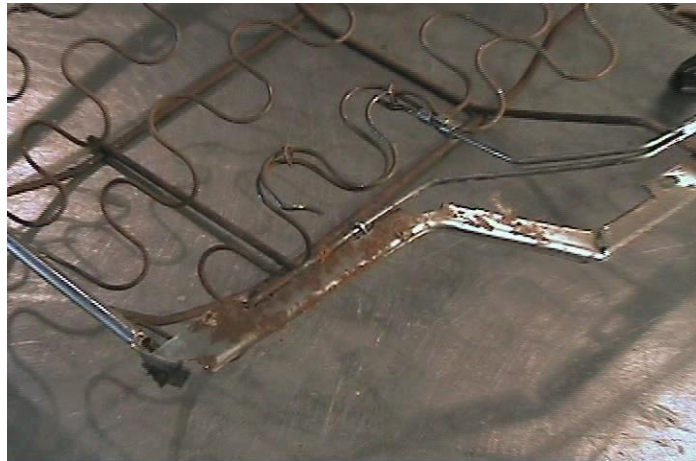
Figure 1 - Rear Seat Frame Modification
