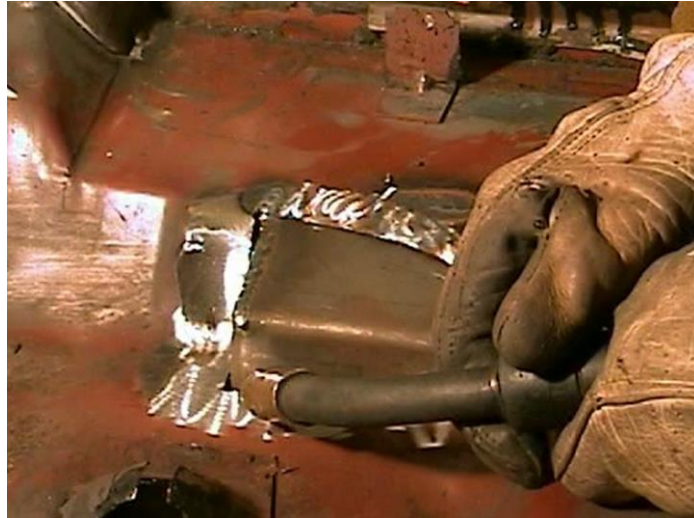
Figure 10 - Welding the Leaf Spring Pocket
