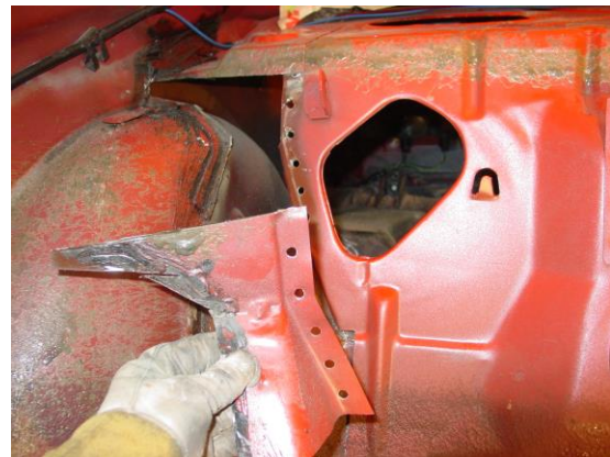
Figure 2 – Seat Support Removed
