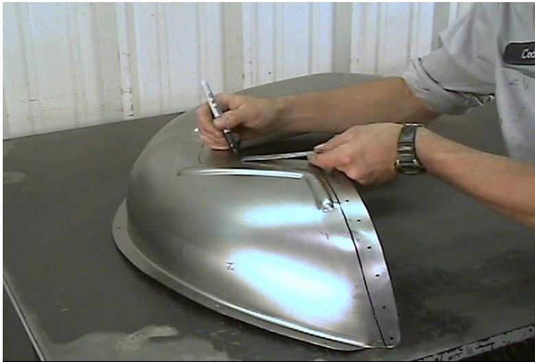
Figure 16 - Mark Tub Mounting Surfaces
