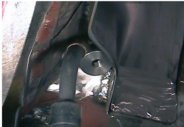
Figure 4 - Weld Seat Belt Mount
