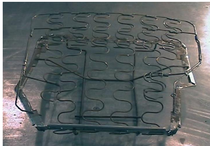
Figure 2 - Narrowed Rear Seat Frame
