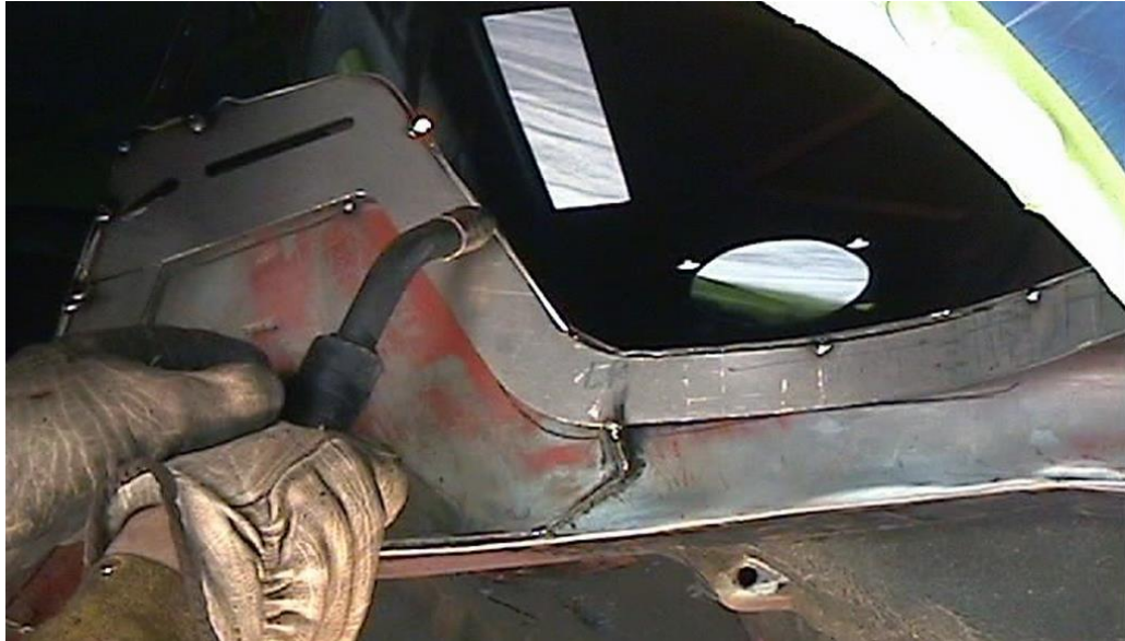
Figure 14 – Tack Weld Tub Flanges
