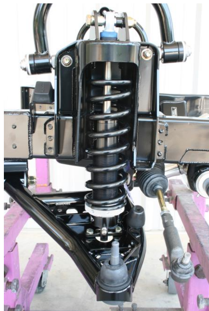
Figure 15 – Installed Coilover View
