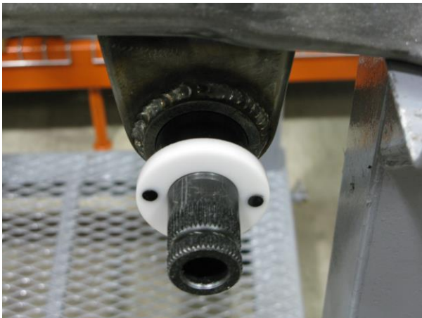
Figure 5 - Installing the Bushing & Anti-Roll Bar
