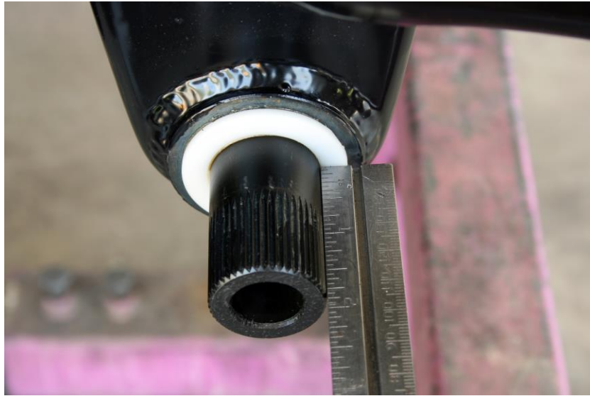
Figure 7 - Measuring the Anti-roll Bar
