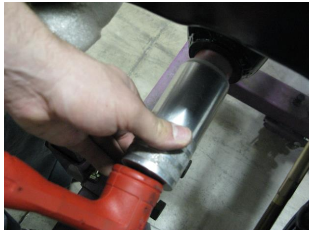
Figure 6 - Fully Installing the Bushings
