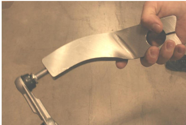
Figure 8 - Pre-assemble the Anti-roll Bar End Links
