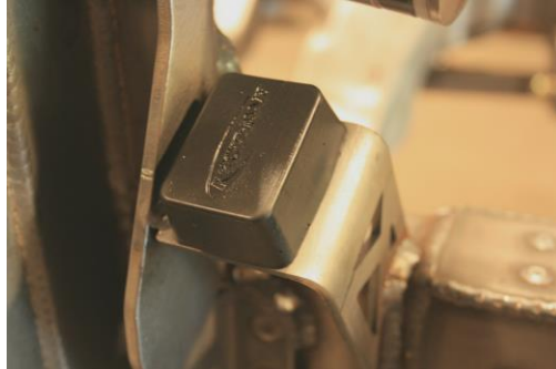
Figure 9 - Installed UCA Bump Stop
