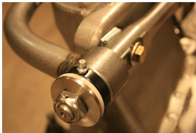
Figure 17 – Installed Upper Control Arm
