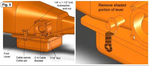
**C-6:** Remove the two transmission oil pan bolts from the left rear corner of the oil pan. Install the cable bracket into position with the two spacers between the pan and the bracket (**See Figure 6**). (If your transmission is equipped with a cast aluminum oil pan, these spacers can be omitted). Install the two supplied 5/16-18 x 1.00" bolts and tighten to 12-13ft.lbs. ft. Do not overtighten as this can damage the pan gasket.
