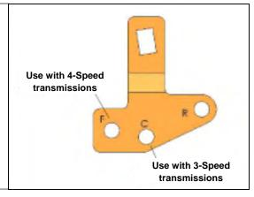
Leave the swivel out of the hole and move the selector lever to Park, all the way forward. Also move the shifter to Park position. (See operation section, page 8). Reinsert the swivel into the hole in the selector lever. Check to see that the swivel will slide freely in and out of the hole in the selector lever in this position. If it does not slip in freely, adjust the swivel slightly until it will slip into the hole in the lever.
