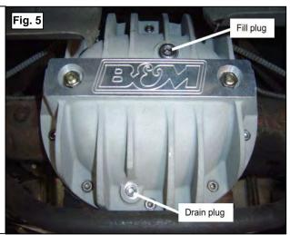
17. Fill with factory recommended gear oil using the B&M Cast Aluminum Rear End Cover fill plug hole (See Figure 5). Add gear oil until oil runs out of the axle housing fill hole.
