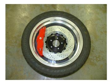
• When installing rotors on any Baer Products be sure to follow the direction of rotation indicated on the rotor hat area with either an arrow, or an "L" for left, or an "R" for right, or both. "L" or left always indicates the driver's side of US spec vehicles. Images shown are "L" left rotors:
