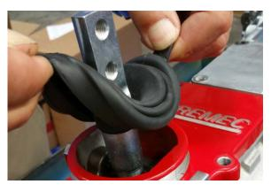
The shifter "body" will be in the in the forward position on the rear T56 shifter cavity. Make sure the pivot ball is positioned into the rear socket and that the white plastic bushing is still in place.
