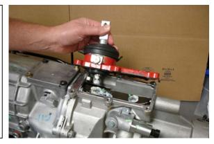
Install the rubber boot onto the Blackjack shifter. Confirm that the rubber boot does not interfere with shifter movement and that the shifter lever movement is not restricted or binding at full travel positions. Failing to do so could result in the shifter popping out of gear and damaging the transmission.
