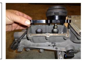
When you are sure your shifter is correctly positioned, apply a new bead of RTV sealer to the lip of the shifter cavity and mount the shifter by re-using the six, 5/16" bolts. Torque the bolts to 20 ft/lbs.
