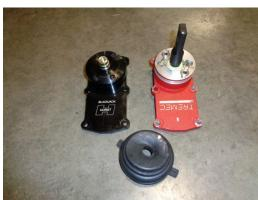
Install the modified boot onto the Blackjack shifter. Confirm that the rubber boot does not interfere with shifter movement and that the shifter lever movement is not restricted or binding at full travel positions. Failing to do so could result in the shifter popping out of gear and damaging the transmission.
