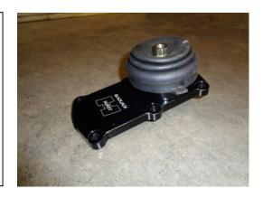
The shifter "body" will be in the forward position on the rear TKO shifter cavity. Make sure the pivot ball is positioned into the forward socket and that the white plastic bushing is still in place.
