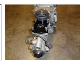
Position the offset stub onto the shifter and make sure that it is offset towards the driver's side as seen in the photo. Secure the offset stick with the provided 3/8"-24 Button Head bolt and washer and torque to 35 ft/lbs.
