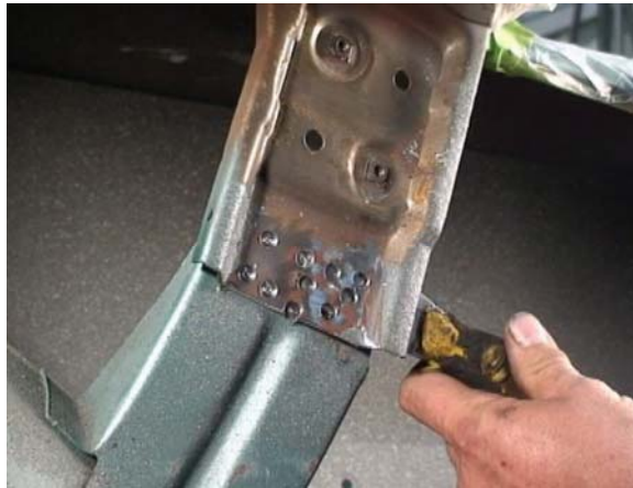
Figure 1. Separating the Passenger Side Trunk Support Flange
