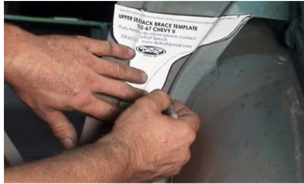
Figure 4. Tracing the Template on the Seatback Brace
