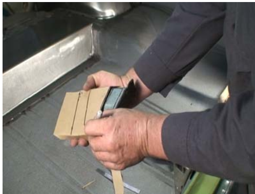
Figure 16. Comparing Cardboard Template to Factory Trunk flange
