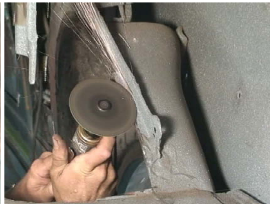
Figure 8b. Cutting the Factory Horizontal Flange
