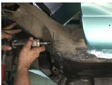
Figure 9a. Mark and Cut Vertical Ends First
