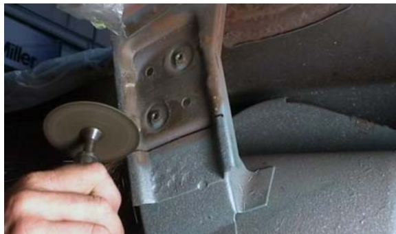
Figure 2. Cutting the Driver Side Trunk Support Flange
