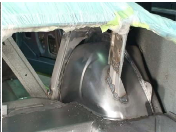
Figure 18b. Finished Passenger Trunk Brace Flange
