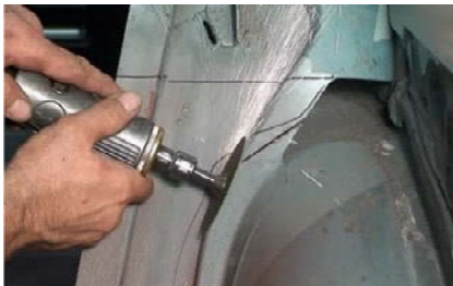
Figure 5a. Cutting the Seatback Brace
