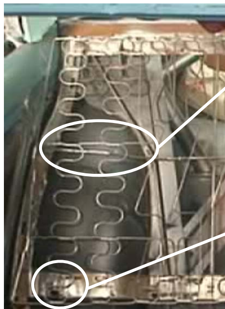
Figure 27a. Finished Modified Seat Frame (Passenger Side)
