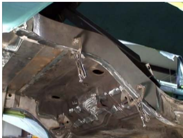
Figure 11. Fitting and Trimming the New Frame Rail Close Out
