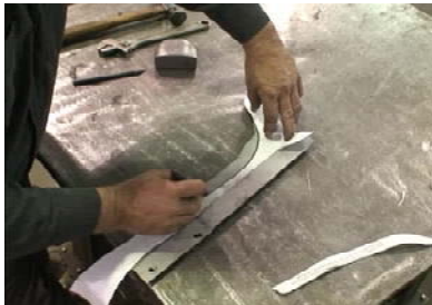
Figure 15a. Trace Template on Brace
