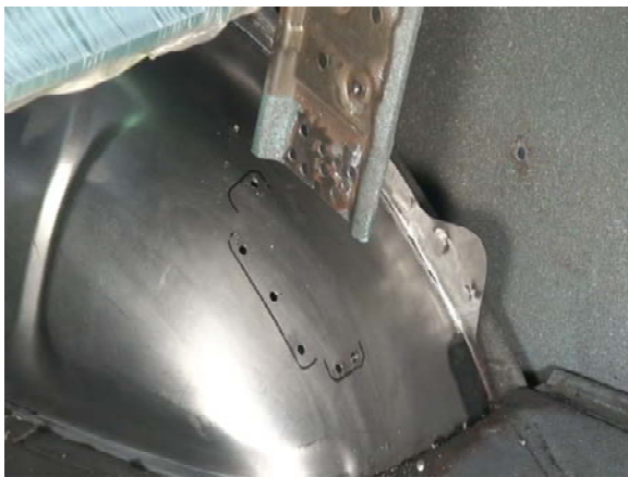
Figure 18a. New Tub Marked for Flange Welding
