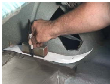
Figure 6a. Tracing the Lower Templates
