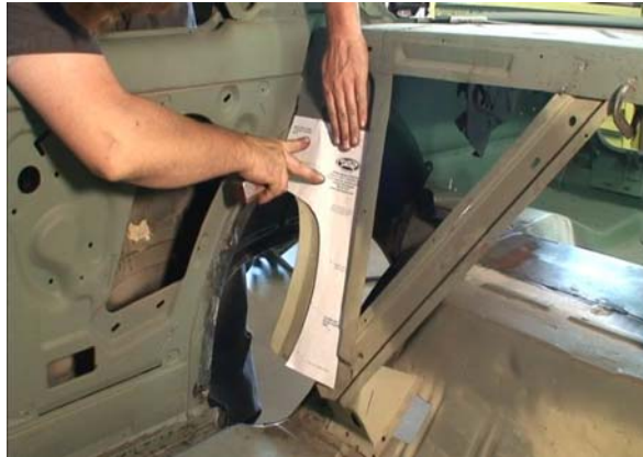
Figure 20. Marking the Upper Seatback Brace
