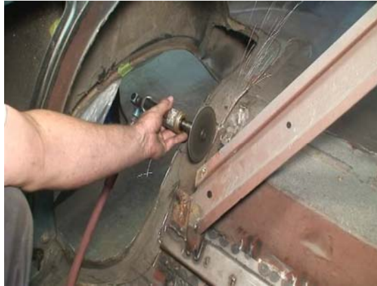
Figure 7. Removing the Previously Traced Floor Pan Section
