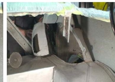
Figure 6c. Removing the Factory Wheel well
