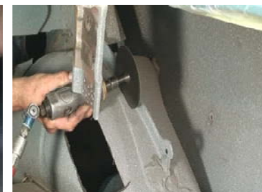
Figure 6b. Cutting the Factory Wheel well
