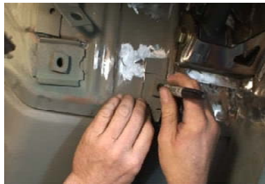
Figure 21b. Mark new Anchor Location
