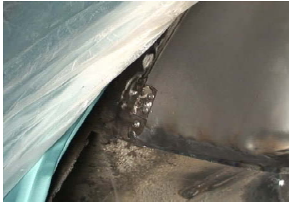
Figure 14b. Rear Lap Flange Bent Into Place
