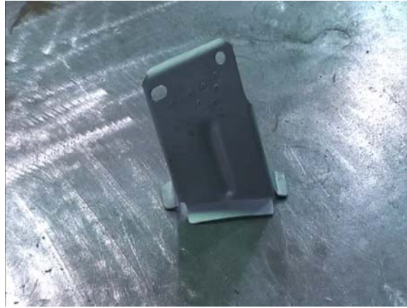
Figure 17. Modified and Primed Factory Trunk Flange
