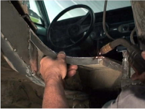
Figure 12a. Fabricating the New Front Flange
