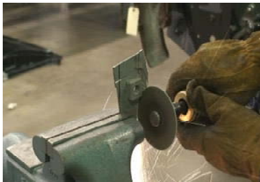
Figure 21a. Mark and Trim Belt Anchors
