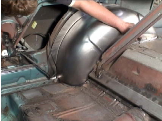
Figure 13a. Marking the Mating Surfaces for Welding
