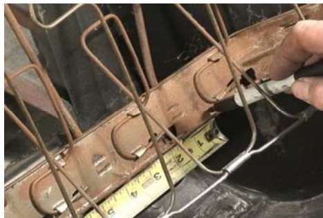
Figure 25. Cut 2" from Top and Bottom Rail
