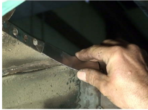
Figure 12b. Fabricating the New Rear Flange
