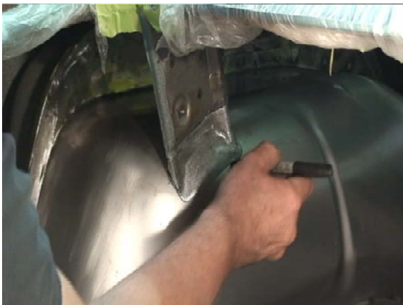
Figure 19a. Marking Driver Side Tub for Welding
