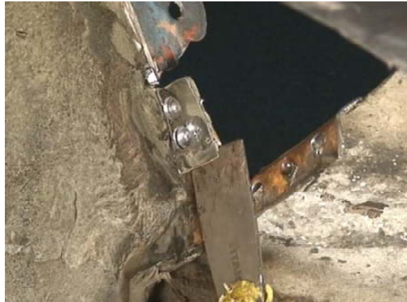
Figure 10b. Removing and Bending Rear Lap Flange
