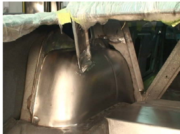
Figure 19b. Finished Driver Trunk Brace Flange
