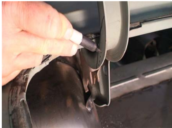
Figure 24. Trimming Trunk Hinges for Clearance
