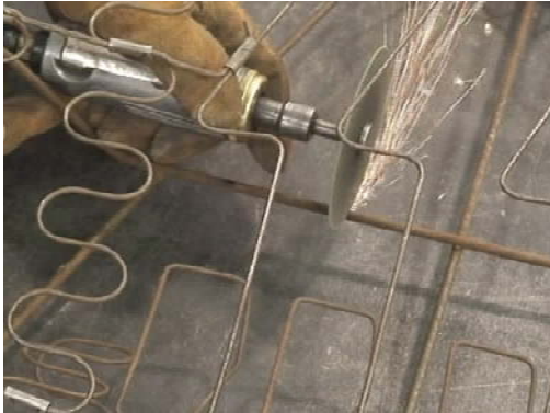
Figure 26a. Cutting the Cross Bar at the 2 ½" Mark
