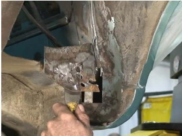
Figure 10a. Removing Forward Lap Flange
