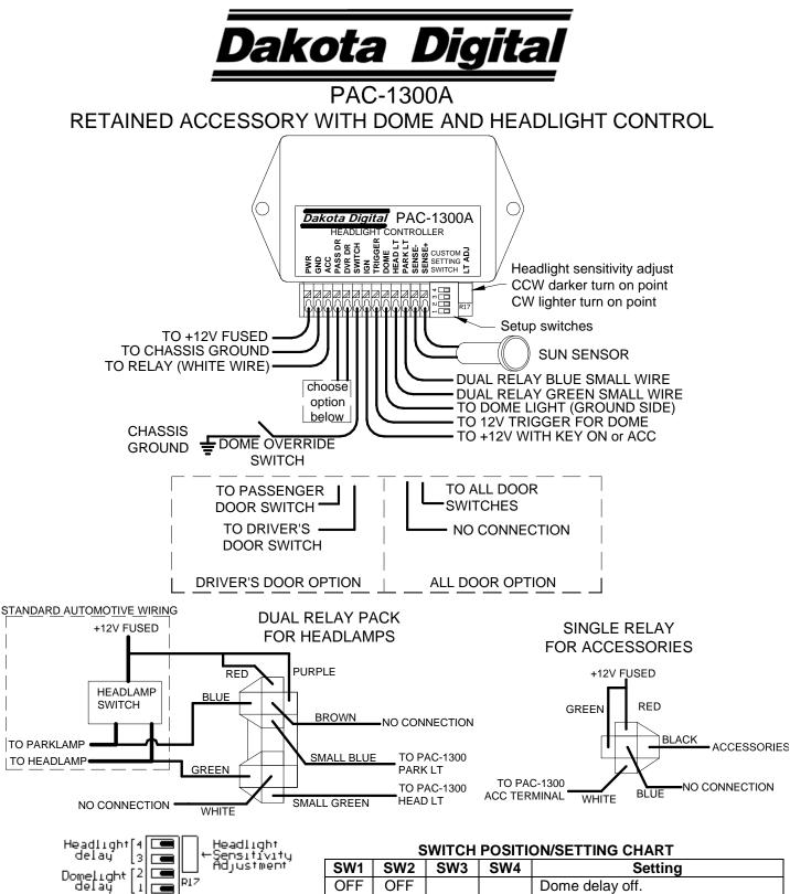
Turning the HEADLIGHT adjustment clockwise increases the sensitivity and will cause the headlights to turn on when it is brighter. Counter clockwise will cause the lights to turn on when it is darker.
