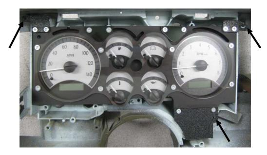
7. Separate the stock lens from the blackout plate; the original lens is not needed. Place the blackout plate over the Dakota Digital gauges while aligning the mounting holes. Attach the VHX system using the five factory screws. Place the included 1/8" white plastic spacer beneath the blackout plate at the lower-most mounting hole before installing the screw (white arrow).
