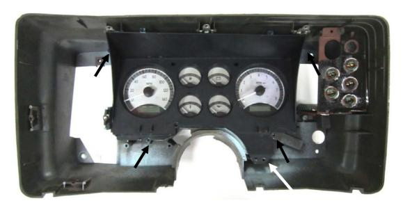
8. If the instrument housing was removed from the dashboard, reinstall, then attach the bezel to the housing with the seven factory screws removed in Step One. Refer to the main manual for wiring instructions to complete the VHX installation.
