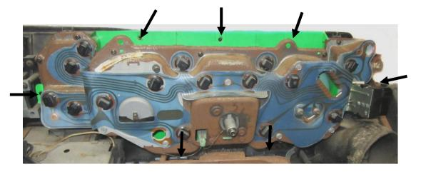
2. With a side cutter, cut the plastic tabs off to remove the factory lens as it won't be reused.
