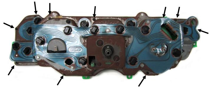
5. With the factory gauges and lenses removed, you will be left with a bare bezel, as shown below.
