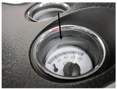
5b. The VHX system should align tightly and the lens should sit flush with the bezel.
