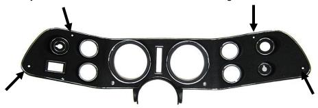
2. Remove the four screws holding the gauges into the dash. These screws will be re-used for the VHX gauge installation.
