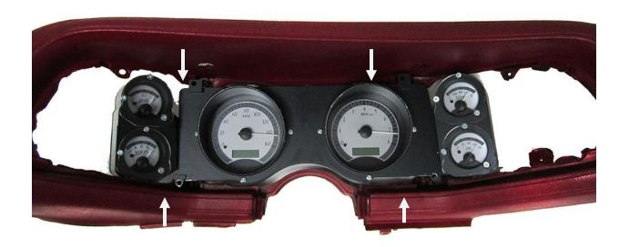
5a. Remove the protective tape from the clear lens and align the bezel with the gauges. Watch carefully as you align the bezel so you don't scratch or damage the lens.
