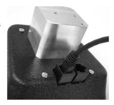
7. Remove the protective lens tape and insert the VHX **speedometer** into the *left* side of the factory housing. You will need to fold the CAT5 cable and route it through the opening where the original indicator lights were mounted in order to get the VHX bezel to sit flush with the housing. As the gauge goes in, route the CAT5 cable through the opening in the bottom of the housing, keeping in mind the cable needs to reach the control box.
