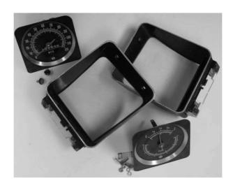
2. Once the original gauge internals have been removed, there are two reflectors (one on each side) inside the housing that need to be removed for clearance of the new VHX gauges (see photo).
