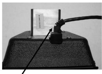
Pre-bend cable to side before installing so unit will sit flush once inserted into dash
