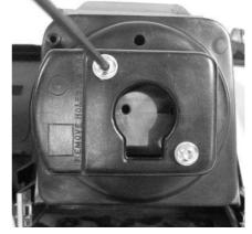
9. To install the tachometer, repeat the steps above, making sure to use the shorter screws and plastic washers. The tachometer uses two 10-32 x 1" screws and two flat nylon washers to secure the gauge.
