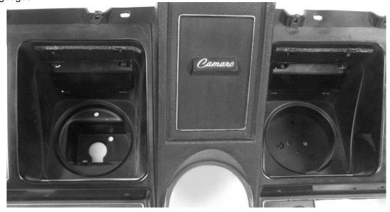
5. Begin with the speedometer installation first; located in the left side opening in the factory dash. Cut three pieces of the supplied foam tape, 2" long. Install foam strips on the top and sides of each opening about ½" down from the face of the housing. This foam provides a cushion where the new VHX cans are installed and forms a tight, rattle-free fit.
