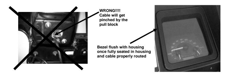
8. Using the two provided **10-32 x 1.5**" screws and **nylon shoulder washers**, secure the speedometer assembly to the housing. Start the screws into the back of the factory housing and into the pull-block on the back of the gauge assembly. Tighten with a 1/8" Allen wrench.
