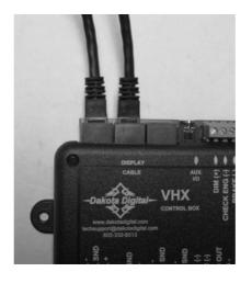
12. Display installation is complete, refer to the main manual for wiring instructions to complete the VHX installation.
